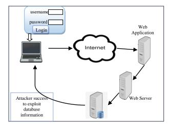
Figure 1. How SQL Injection Attack Works
